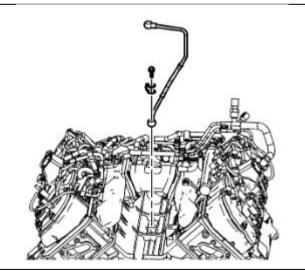
5. Install the turbocharger lower heat shield.
